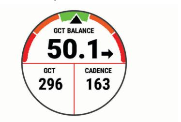
**REMEMBER:** Ground contact time balance is available only if you are using a compatible running dynamics accessory.
